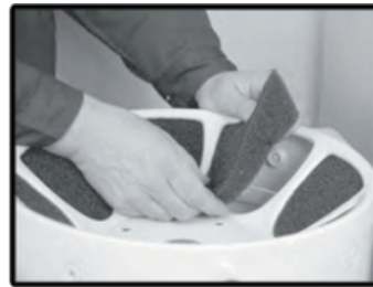
Remove old silencer and fit new silencer.
