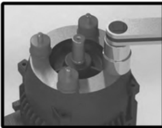
Remove old motor mounts and replace with new motor mounts. Tighten mounts to 8Nm.
