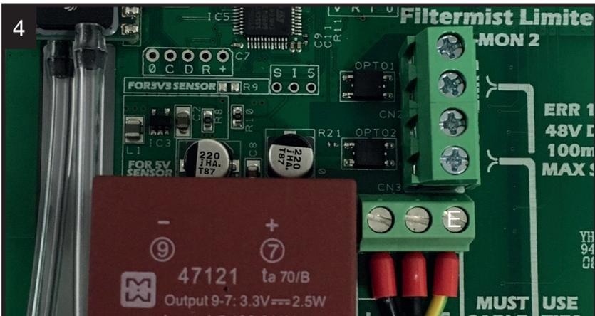
The F Monitor 2 comes with 3 metres of cable already prewired. If a longer length is needed ensure it is connected as shown above.
