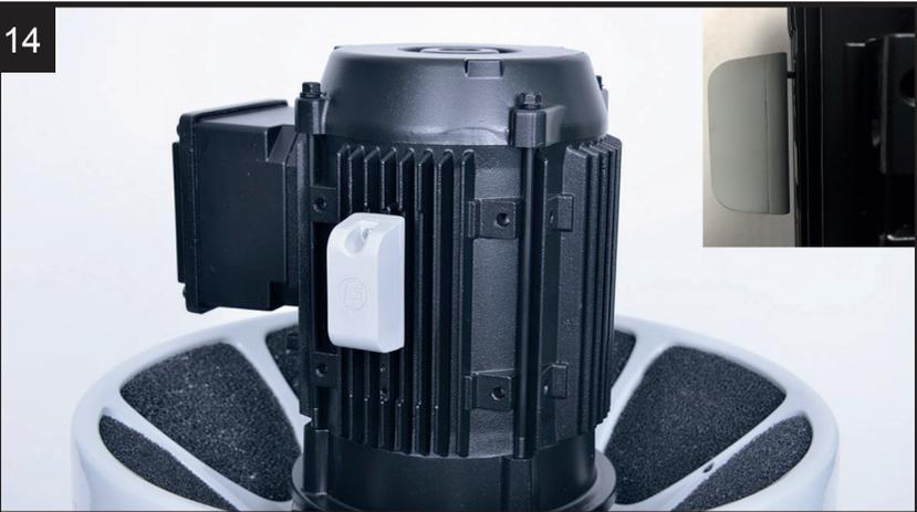
Optional: Use the hole on the side of the motor to attach the sensor, ensure that the sensor is secure and rigid - there must be a gap between the motor and the sensor. It should not be loose, otherwise the vibration reading will not be correct.
