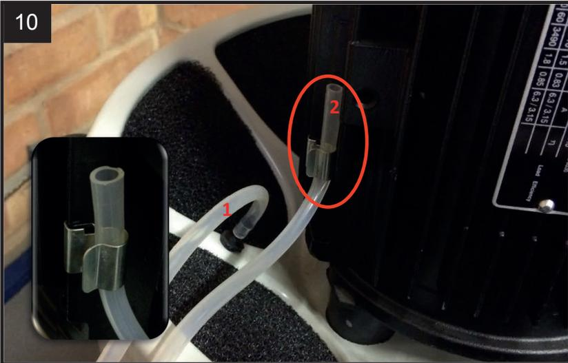
Attach motor clip to motor vane and clip tube 2 into position (tube should point vertically upwards)
