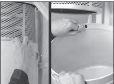
(4) Clean area where top and bottom of case join & clean drain hole.
