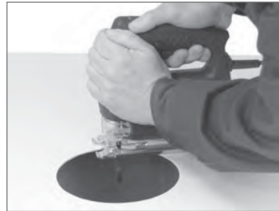
(4) Cut extraction hole in machine enclosure.
