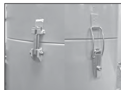
(9) Re-assemble unit. IMPORTANT! Ensure safety latch and clip are securely fastened.
