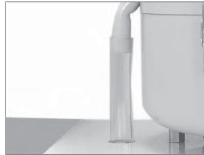
(4) Fit oil return tube and position tube to drain oil back to machine enclosure, sump or collection vessel.
