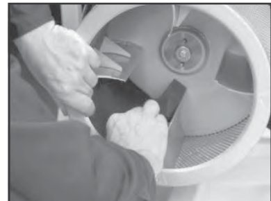
(6) Fit new drum pads.
