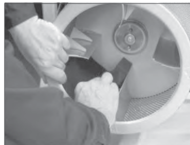
(8) Fit new drum pads.
