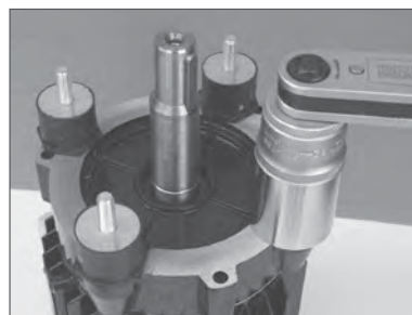
(11) Remove old motor mounts and replace with new mounts. Tighten mounts to 8Nm.
