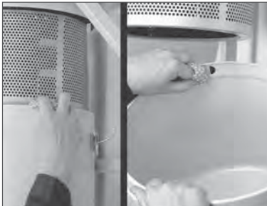
(4) Clean area where top and bottom of case join & clean drain hole.
