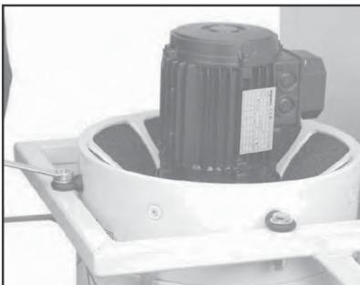
(5) Position unit in stand and secure unit with bolts (supplied with unit).
