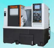
Mazak QTP100S, QSM100, QSM150 CNC Lathe
